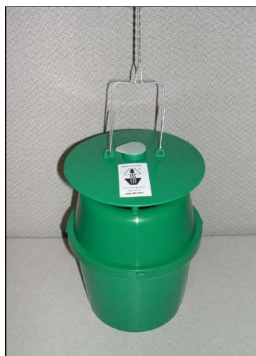
Figure 8: Hanging trap from top using wire hangar.
